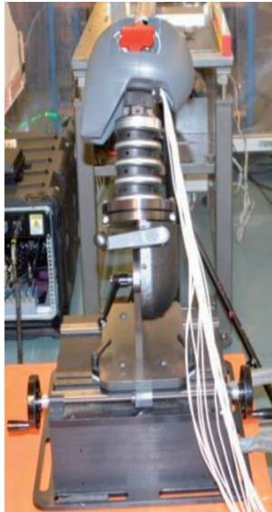
**Figure 4.-** Ballistic Load Sensing Head form
