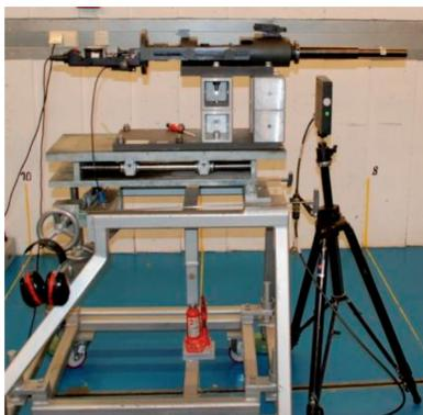
**Figure 2.-**Universal receiver with interchangeable barrel
