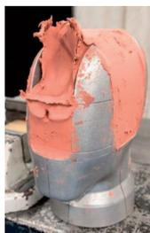
**Figure 9.-** Army clay head form with Weible clay, after a test.
