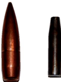
**Figure 1.-** 7.62x39 mm M43 and its core.
